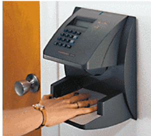
Access Control Terminal
